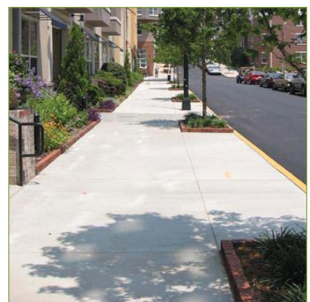
Pedestrian facilities seen here include appropriate sidewalk dimensions, pavement conditions, and vegetation buffer
