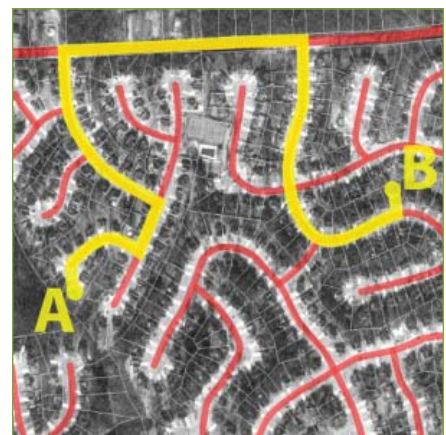
A dendritic street system allows fewer choices of travel, with a trip from A to B at a distance of one mile
