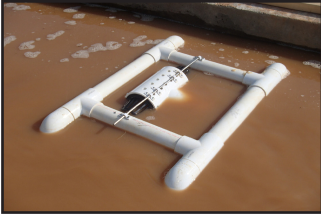
Figure 6-31.1. Floating skimmer of a different design.
