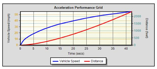
Acceleration Performance: TIME TO ACCELERATE ON A 0.00% GRADE TO 55.0 (MPH) IS 42.20 (SECS)
